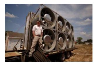
University of Florida wind engineering researcher Forrest Masters stands on a newly completed, fully portable hurricane wind simulator on May 29, 2007.
