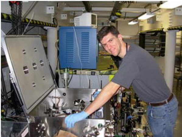
Chris Sears leans over the experimental chamber where researchers hope to accelerate electrons with laser light.
