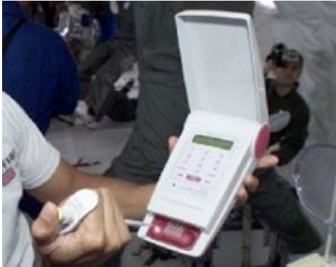
LOCAD-PTS, a handheld biological laboratory for space travel.
