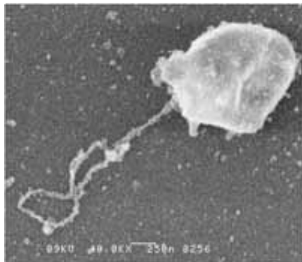
This scanning electron micrograph of Dehalococcoides (Dhc) bacteria shows the GT strain of the microbes that dechlorinated PCB contamination in lab tests. Credit: Georgia Institute of Technology
