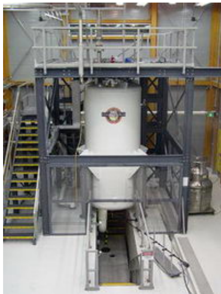
900 MHz Magnet at Florida State University National High Magnetic Field Laboratory. Courtesy of NHMFL, Florida State University, Tallahassee, Fla.
