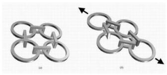
The micromachined chain mail fabric is made of links and rings, which can slide against each other to create a flexible fabric. Credit: Engel, et al.
