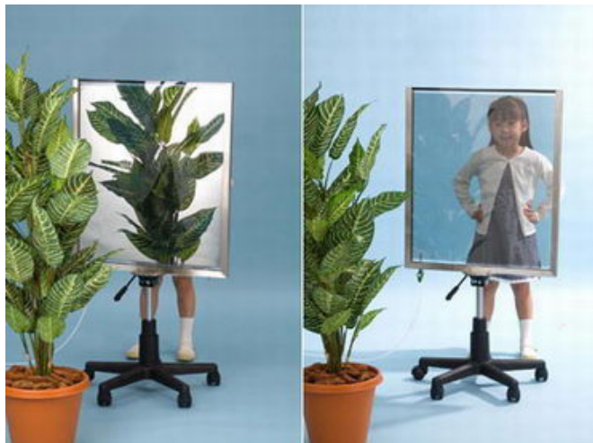
Switchable mirror that turns into a color-neutral transparent state. Credit: AIST
