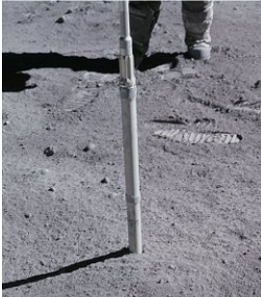
Apollo 16 astronaut Charlie Duke (feet shown) drives a core sample tube into the lunar regolith.
