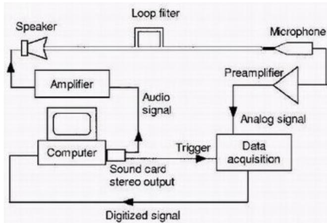
In this schematic of the acoustical test system, the scientists could create superluminal group velocity of sound waves, as well as negative group velocity. In the latter case, the peak of the output pulse traveling through the loop filter exited the filter before the peak of the input pulse had reached the beginning of the filter. Image credit: Bill Robertson, et al.
