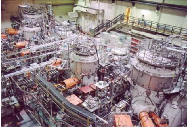
The GAMMA 10 tandem mirror at the University of Tsukuba in Japan is the world's largest tandem-mirror plasma-confinement experimental device. In the future, such a device may use the cooling concept presented in this study by Nathaniel Fisch. Image credit: Teruji Cho, University of Tsukuba Plasma Research Center.
