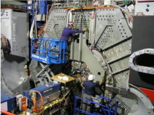
Workers install a yoke on the front of the BaBar detector to help carry the load of the electromagnetic calorimeter while the muon system is upgraded. Credit: SLAC
