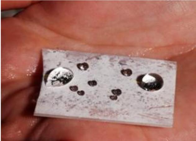
Close-up image shows water beading up on a coating modeled after the surface of lotus plant leaves. Credit: Gary Meek / Georgia Tech Photo
