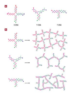
DNA chains that attach to one another along part of their length can self-assemble into branching structures including crosses, T's and Y's. In the presence of enzymes that connect the open ends to one another, these shapes combine into larger structures with many small openings, creating a sponge-like material called a hydrogel. Credit: Molecular Bioengineering Lab/Cornell University
