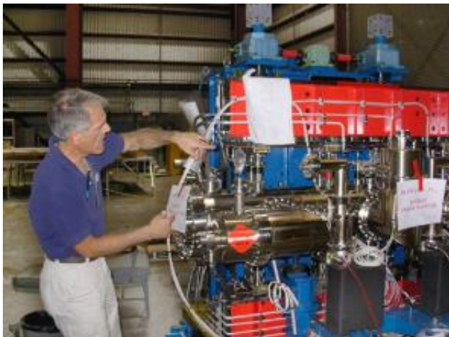
Beamline development group leader Tom Rabedeau explains the design of the in-vacuum undulator for the new Beamline 12.
