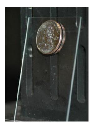
Using only a sheet of micro-fiber array on its back without any traditional adhesive — a quarter clings to a glass slide inclined at a steep, 80-degree angle. Credit: Photo courtesy of the Fearing Group, UC Berkeley
