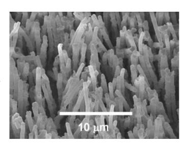
long, 0.6 micron diameter polymer fibers. Scale bar represents 10 microns. Credit: Image courtesy of the Fearing Group, UC Berkeley
