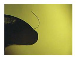
Microscopic flash photography shows a carbon fiber 5 microns in diameter bending nearly 90 degrees while driven to oscillate at 33.4 kHz. The combined flexibility and durability of carbon fibers suggest many uses in microelectromechanical (MEMS) devices, including use as springs and as supports for vibrating objects. Credit: Thompson Lab/Cornell University
