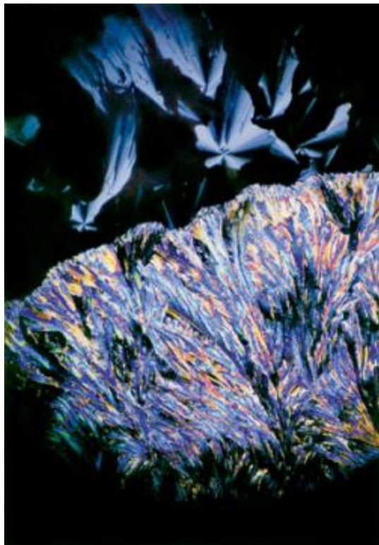
Micrograph of a metal-rich, zinc chloride-based liquid crystal.
