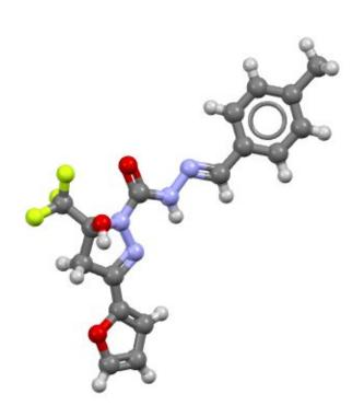
An example of the 1,800 medically relevant crystal structures in the CSD that were identified as conglomerates. These structures have spontaneously enriched chirality on crystallization, presenting more starting materials that medicinal chemists could use in drug design. Credit: The Cambridge Crystallographic Data
