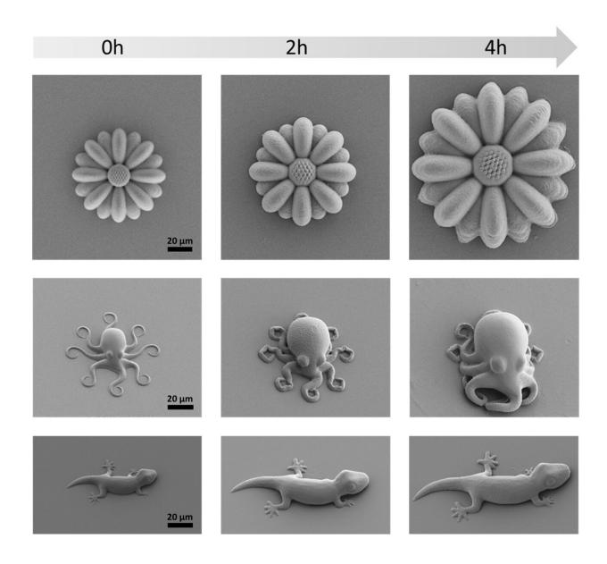
Smart polymers with "life-like" properties: due to dynamic chemical bonds the
