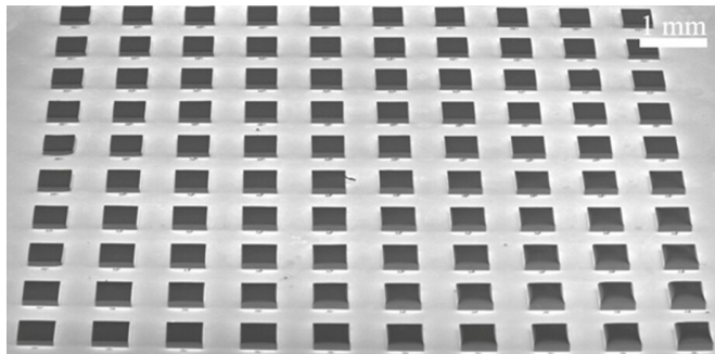
SEM micrograph of a cuboid parameter sweep comprising 10 x 10 elements fabricated via TPP from the photoresist IP-Q. Credit: The Authors doi: 10.1117/1.JOM.2.3.033501.
