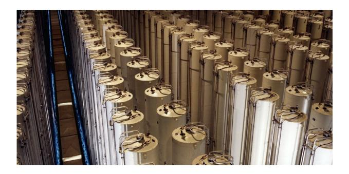
A cascade of gas centrifuges at a U.S. enrichment plant in Piketon, Ohio, in 1984. Iran is using similar technology to enrich uranium. Credit: <u>U.S.</u> <u>Department of Energy</u>
