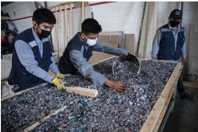
Men work at a factory that recycles used clothes discarded in the Atacama desert for housing insulation panels, in Alto Hospicio, Iquique, Chile.
