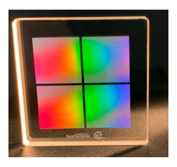
Researchers developed a new fast and energy-efficient laser-writing method for producing nanostructures in silica glass. They used the method to record 6 GB
