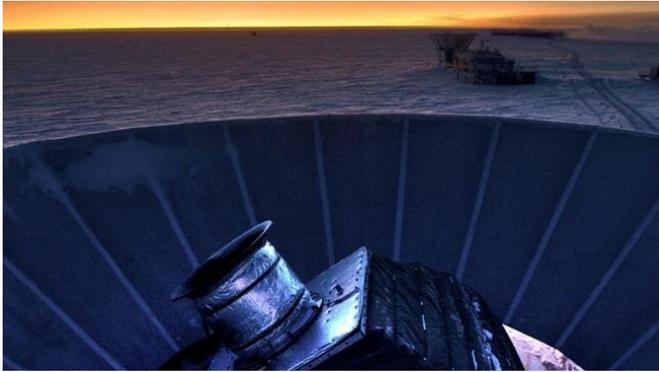
The BICEP3 telescope located at the Amundsen-Scott South Pole Station in Antarctica. (The metal skirt around the telescope shields it from reflected light from the surrounding ice.) New results analyzing BICEP3 data together with earlier data and the datasets from space missions have improved previous constraints on the kinds of models of inflation that could describe the earliest moments of the universe. Credit: Harvard-Smithsonian Center for Astrophysics
