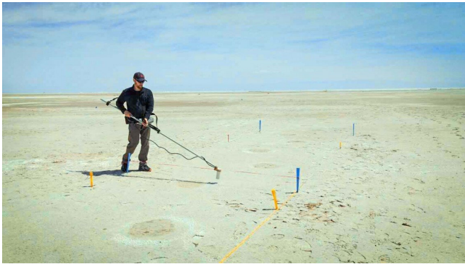
Thomas Urban conducts a magnetometer survey of mammoth footprints at White Sands. Credit: David Bustos / Cornell University
