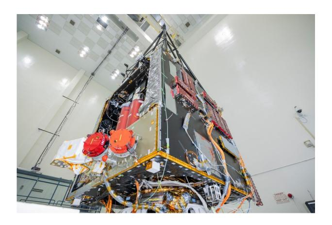
NASA's Psyche spacecraft is photographed in July 2021 during the mission's assembly, test, and launch operations phase at JPL. Hall thrusters will propel the spececraft to its target in the main asteroid belt. Credit: NASA/JPL-Caltech
