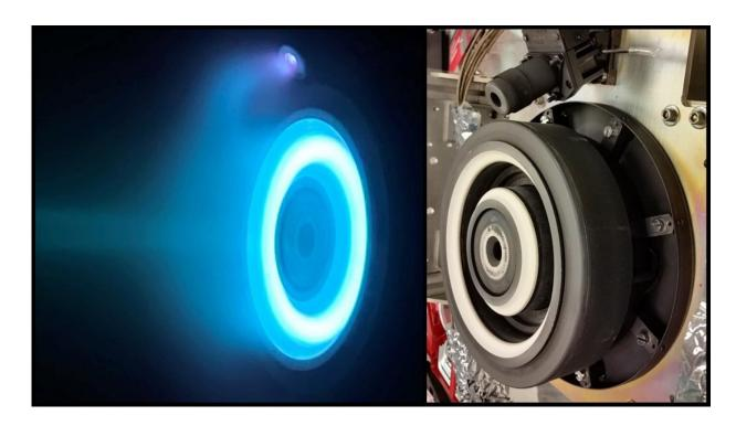
At left, xenon plasma emits a blue glow from an electric Hall thruster identical to those that will propel NASA's Psyche spacecraft to the main asteroid belt. On the right is a similar non-operating thruster. Credit: NASA/JPL-Caltech
