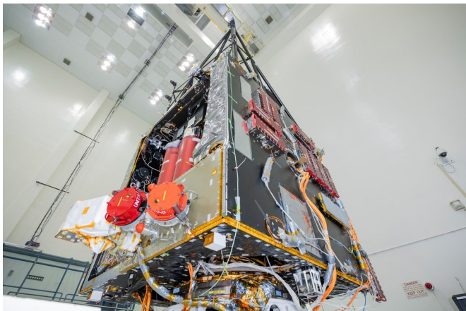
NASA's Psyche spacecraft is photographed in July 2021 during the mission's assembly, test, and launch operations phase at JPL. Hall thrusters will propel the spacecraft to its target in the main asteroid belt. Credit: NASA/JPL-Caltech
