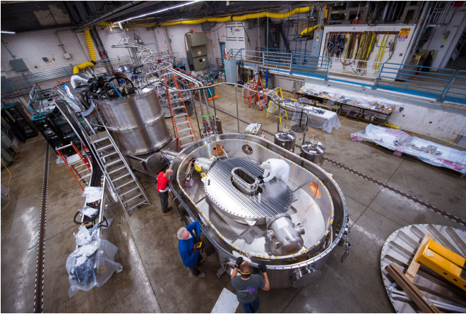
Collaborative team working on the magnet inside the test stand housed at MIT. Research, construction and testing of this magnet has been the single largest activity for the SPARC team, which has grown to include 270 members. Credit: Gretchen Ertl, CFS/MIT-PSFC, 2021
