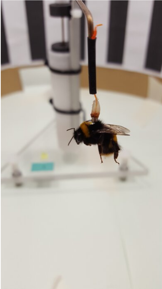
A bumblebee attached to a flight mill. Credit: Daniel Kenna / Imperial College London
