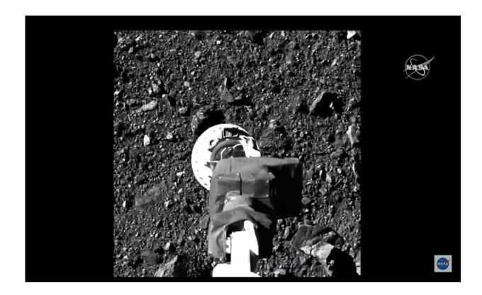
A NASA video frame handout image shows the robotic arm from NASA spacecraft OSIRIS-REx collecting samples from the asteroid Bennu.
