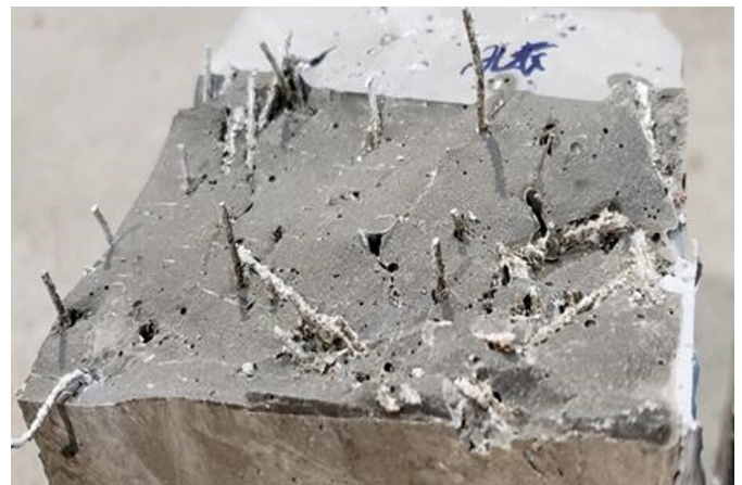
Prototype of fusible metal fiber-reinforced concrete. Credit: Tokyo Institute of Technology
