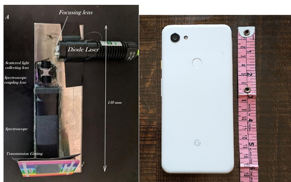
Photo showing relative size of spectrometer (left) and cellphone (right and at the lower end of the spectrometer). Credit: Peter Rentzepis
