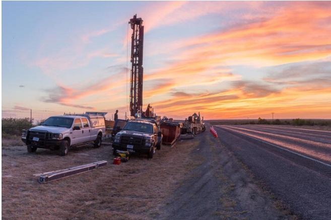
A coring and geophysical well-logging operation rises beside U.S. Route 90 in Kinney County, Texas. Credit: Stanley T. Paxton, U.S. Geological Survey
