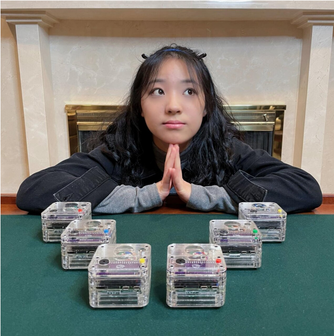
Vivien He with her earthquake early warning devices to be deployed across Los Angeles. Credit: Vivien He
