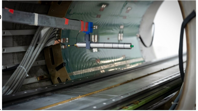
Calibration probe inside of the solenoid magnet at Argonne's 4 Tesla Solenoid Facility. Credit: Mark Lopez, Argonne National Laboratory
