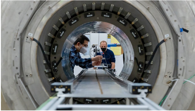
Argonne's Ran Hong (left) and Simon Corrodi (right) installing the calibration probe at the 4 Tesla Solenoid Facility. Credit: Mark Lopez/Argonne National Laboratory
