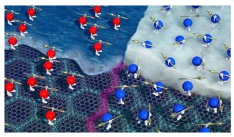
Pomeranchuk effect in magic angle graphene, revealing an exotic transition between two phases: A (Fermi) liquid phase, where the spatial positions of electrons are disordered but their magnetic moments (arrows) are perfectly aligned, and a solid-like phase where the electrons are ordered in space but their magnetic moments are fluctuating freely. Counterintuitively, the liquid phase transforms to the solid-like phase upon heating. Credit: Weizmann Institute of Science
