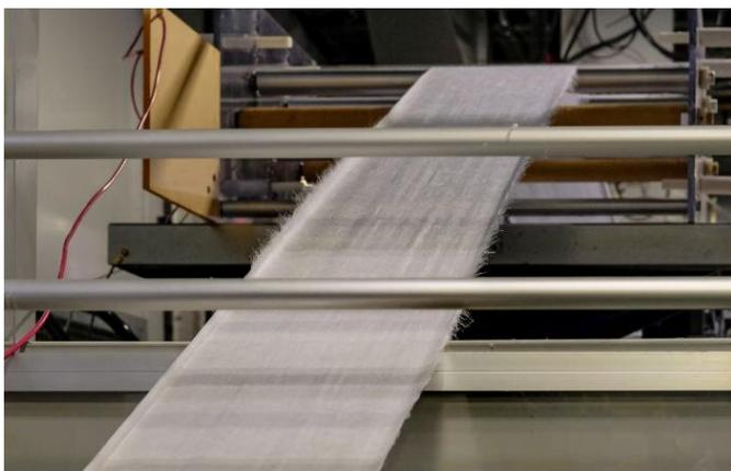
The N95 filter material — made of polypropylene — was produced on the melt-spinning precursor line at DOE's Carbon Fiber Technology Facility at ORNL. Paranthaman used neutrons and microscopy and analyzed three different blends of the material to determine the characteristics necessary for enhancing filter efficiency. Credit: ORNL/U.S. Dept. of Energy
