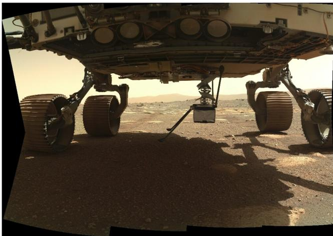
Ingenuity (shown on the surface of Mars behind the Perseverance rover) will perform tests of its rotors and motors over the coming days ahead of its first flight attempt, scheduled no earlier than April 11
