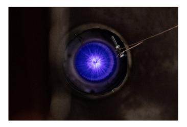
Electron beam irradiation with a dose ? 5 kGy is sufficient for full disinfection of the egg surface. Credit: UrFU / Ilya Safarov
