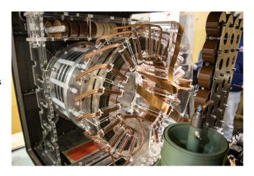
Irradiation experiments were carried out by the means of the URT-0.5 accelerator. Credit: UrFU / Ilya Safarov
