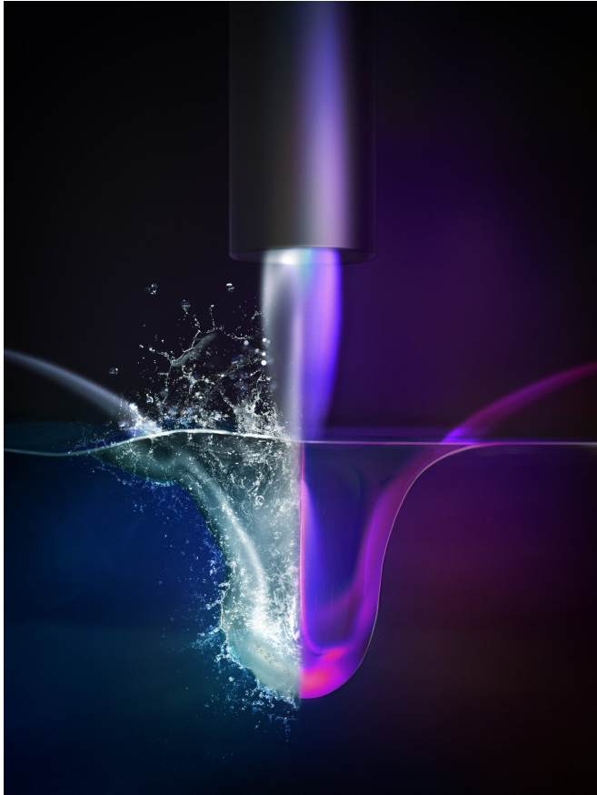
Cavity formation at the water's surface subjected to a neutral helium gas jet (left) and a weakly ionized helium gas jet (right). Credit: The Korea Advanced Institute of Science and Technology (KAIST)
