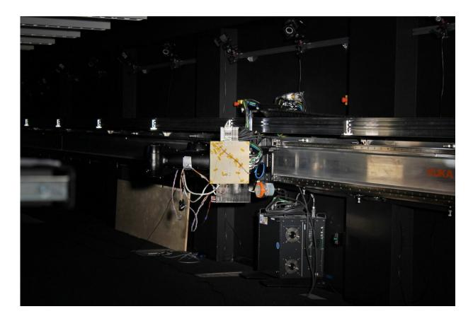
The reduced version of the LED target plate for Proba-3 vision-based sensor system testing, mounted on the robotic arm in the GRALS facility. Credit: ESA
