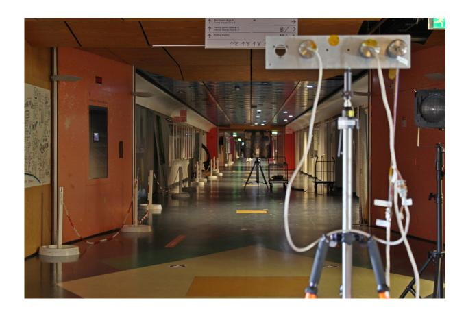
Pre-test with the target at 15m distance from the camera to check good functioning of Proba-3's vision-based sensor system. The testing for the formation flying mission took place in ESTEC's 230-m-long main corridor. Credit: ESA
