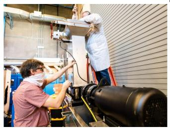
Known commonly as the "Muffin Monster," this customized industrial grinder at Pacific Northwest National Laboratory is used to shred biomass, including food waste, to create a slurry that can be pumped into a reactor that converts it to energy-rich biofuel that could be used in fuel blends that take the place of conventional fossil fuels. Credit: Andrea Starr | Pacific Northwest National Laboratory
