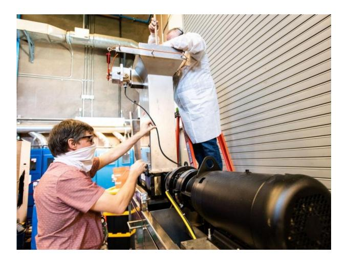
Known commonly as the "Muffin Monster," this customized industrial grinder at Pacific Northwest National Laboratory is used to shred biomass, including food waste, to create a slurry that can be pumped into a reactor that converts it to energy-rich biofuel that could be used in fuel blends that take the place of conventional fossil fuels. Credit: Andrea Starr | Pacific Northwest National Laboratory
