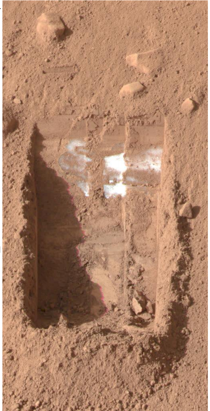
NASA's Phoenix Mars Lander shows the trench, called 'Dodo-Goldilocks,' lacking lumps of ice seen previously. The ice had sublimated, a process similar to evaporation, over the course of four days. Credit: NASA/JPL-Caltech/University of Arizona/Texas A&M University
