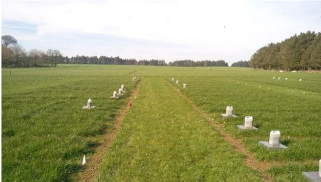
Experimental plots with greenhouse gas measurement chambers in Teagasc Johnstown Castle Research Centre. Credit: Teagasc
