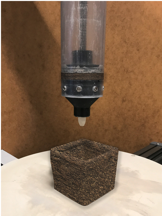
3-D printing of a sample based on mycelium. Credit: Fraunhofer UMSICHT
