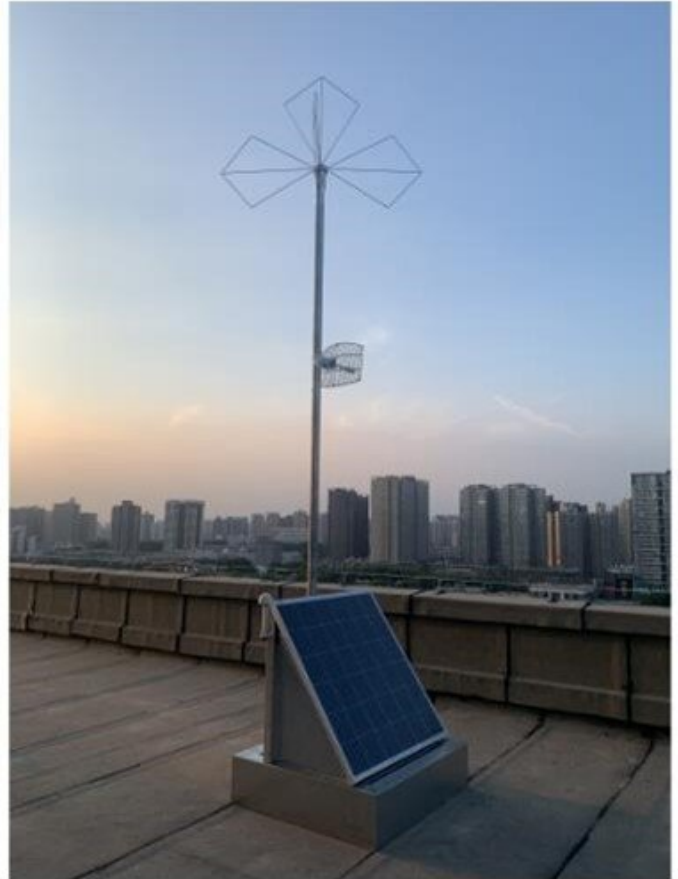
A prototype data collector and transceiver for the GRAND system. Credit: Sijbrand de Jong / GRAND Collaboration
