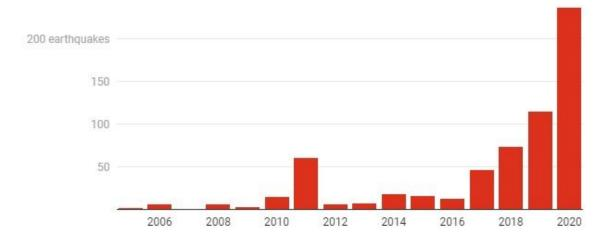
Earthquakes were rare in West Texas before the hydraulic fracturing boom. The chart shows the number of earthquakes above magnitude 2.5 between 2005 and 2020.
