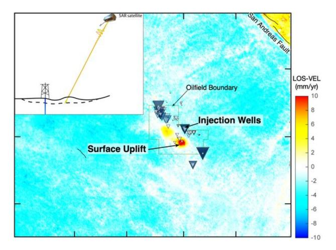
Satellite data shows the ground rising as much as 1.5 centimeters per year in parts of the San Ardo oil field. The line-of-sight velocity (LOS-VEL), as viewed from the satellite, shows how rapidly the ground surface is rising. Credit: Thomas Goebel/University of Memphis
