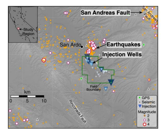
The stresses from injecting water can trigger earthquakes several miles from the well itself. The blue triangles scale with each well's injection rate. Credit: Thomas Goebel/University of Memphis, <u>CC BY-ND</u>
