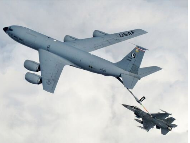
Space battles will likely be between satellites, and refueling will not be an option. In this image, an F-16 is refueling from a KC-135 Stratotanker. Credit: By U.S. Air Force
