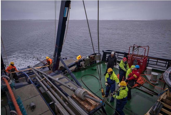
Rigging gravity corer on the deck of icebreaker Oden on SWERUS-C3 expedition 2014. Credit: Björn Eriksson
