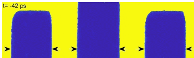
Numerical simulations on the EM wave propagation dynamics in two interdigitated combs. (A) Typical snapshots of the simulated electric field distribution (projected in the x-y plane at the mid-comb thickness) around the active and ground tines at different delay times (movie S2). The arrows indicate the direction of the electric fields with encoded color for the field strength. (B) Plots of the electric fields with encoded color for the field strength. (C) Plots of the electric field Ex as a function of time at three representative positions (P1, P2, and P3) around a ground tine. The field strength near the corner of the tine is stronger than other positions, indicating a local field enhancement near the corner. (D) Plots of the corresponding electric field Ey as a function of time at the three representative positions. The field strength of Ey at
