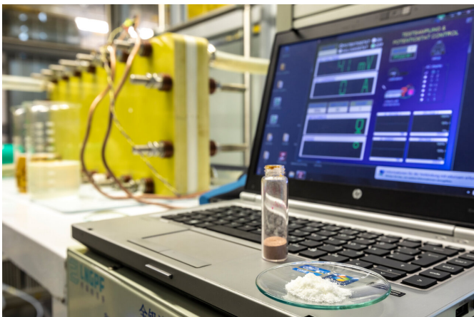
Tests at TU Graz with a 3 kilowatt hour prototype and with vanillin-based electrolytes proved the effectiveness of the new process. Credit: Lunghammer - TU Graz
